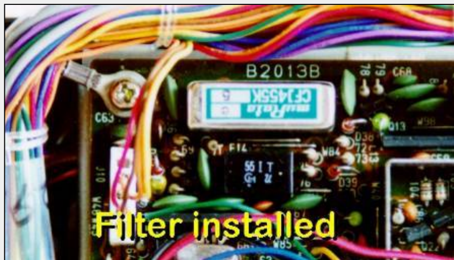
Picture 1 - The Murata filter fitted to the "Main Unit" PBA after the modification.
